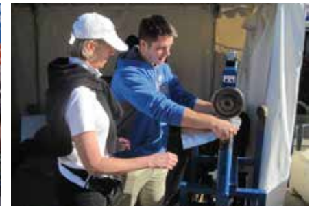
Sean teaching Diane Fitzgerald how to shape metal using an English Wheel, at Penn College's display booth in Hershey, PA.
